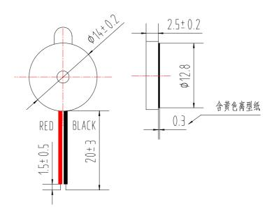
\*Unit: mm; Tolerance: ±0.5mm Except Specified
